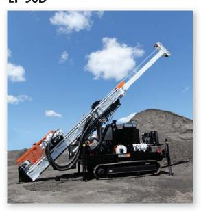
GENERAL SPECIFICATIONS LF-90D, with its compact design and deeper drilling capacity along its competitors, is capable of completing wire-line diamond core drill holes. Crawlers enable LF-90D to move along rugged terrain.
