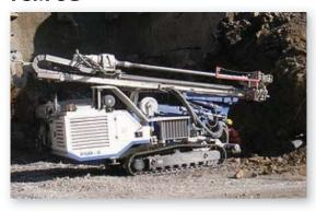
Max. Diameter (mm): 60-260 Engine Power (kw): 103 Max. Depth (m): 320 Max. Tork (Kn.M): 10 Weight (ton): 9
